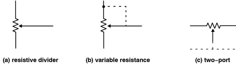
Figure 6. Potentiometer Configuration
