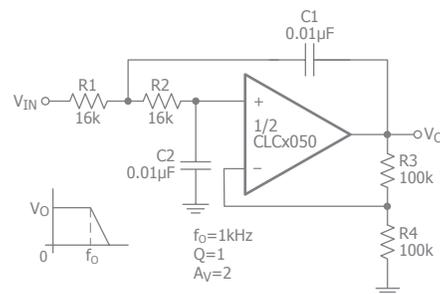
Figure 22. DC-Coupled Low-Pass Active Filter
