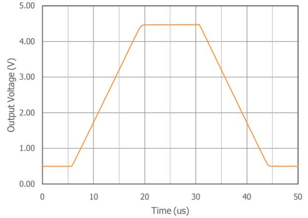
Small Signal Pulse Response at  $V_S = 5\text{V}$
