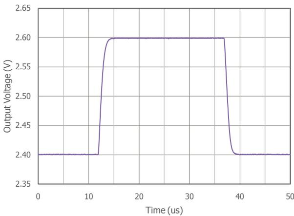
Large Signal Pulse Response at  $V_S = 5\text{V}$
