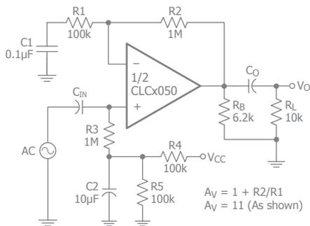
Figure 19. AC-Coupled Non-Inverting Amplifier
