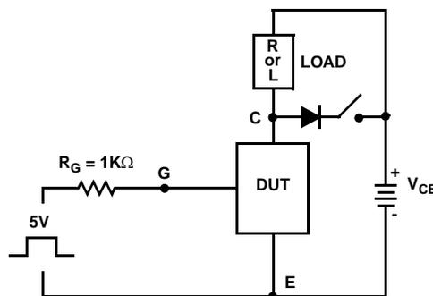
**Figure 18. t<sub>ON</sub> and t<sub>OFF</sub> Switching Test Circuit**
