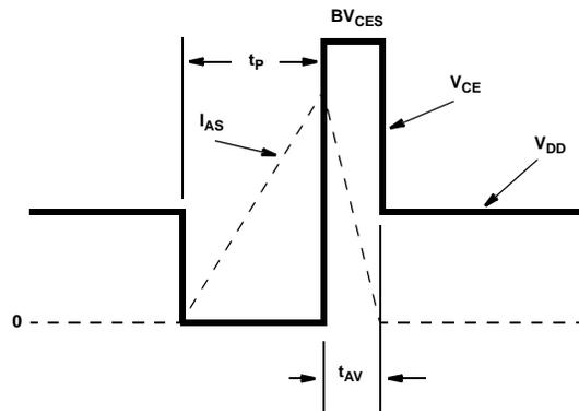
**Figure 20. Energy Waveforms**
