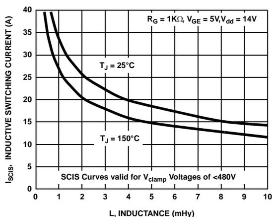
Figure 2. Self Clamped Inductive Switching Current vs Inductance
