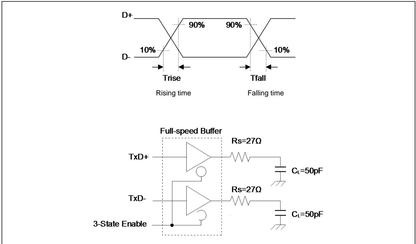
\*6: USB Full-speed connection is performed via twist pair cable shield with  $90 \Omega \pm 15\%$  characteristic impedance (Differential Mode).
