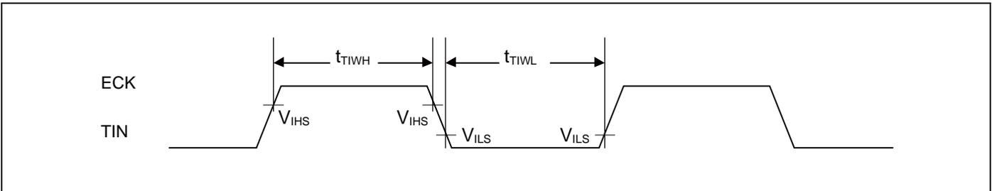
**Trigger input timing**
