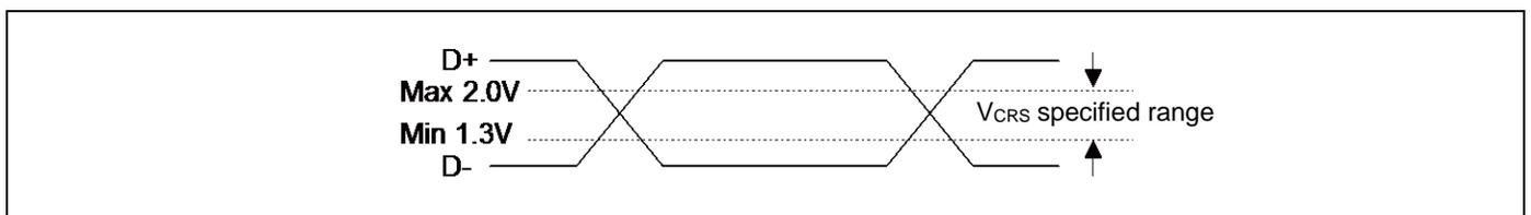
\*5: They indicate rising time ( $T_{rise}$ ) and falling time ( $T_{fall}$ ) of the full-speed differential data signal. They are defined by the time between 10% and 90% of the output signal voltage. For full-speed buffer,  $T_r/T_f$  ratio is regulated as within  $\pm 10\%$  to minimize RFI emission.
