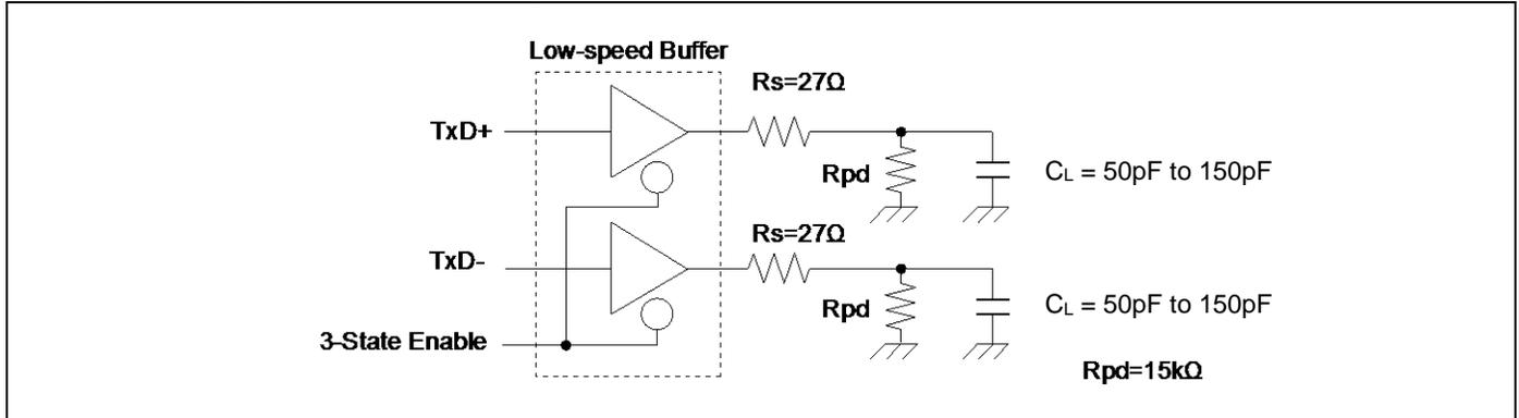
**Low-Speed Load (Downstream Port Load) - Reference 2**
