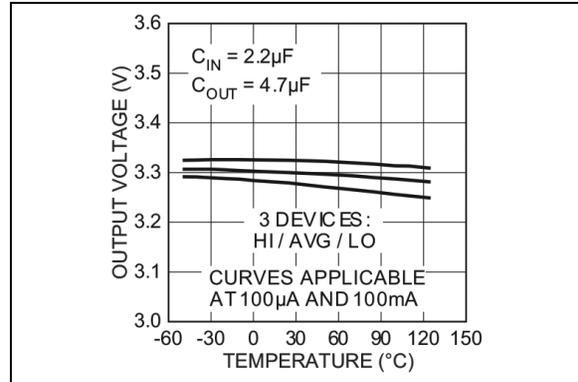
**FIGURE 2-10:** Output Voltage vs. Temperature (3.3V Version).
