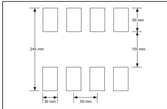
**FIGURE 4-4:** Minimum Recommended 8-Lead SOIC PCB Pads Size.
