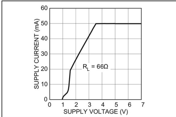
**FIGURE 2-19:** Supply Current vs. Supply Voltage (3.3V Version).
