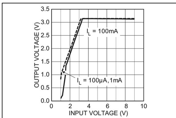
**FIGURE 2-3:** Dropout Characteristics.
