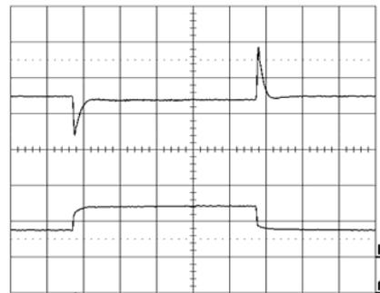
Output voltage response to load current step-
