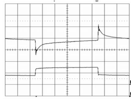
Output voltage response to load current step-
