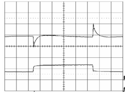
Output voltage response to load current step-
