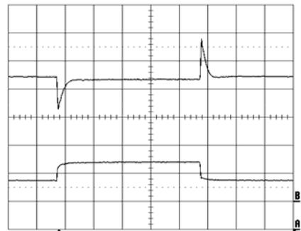
Output voltage response to load current step-
