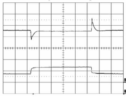
Output voltage response to load current step-
