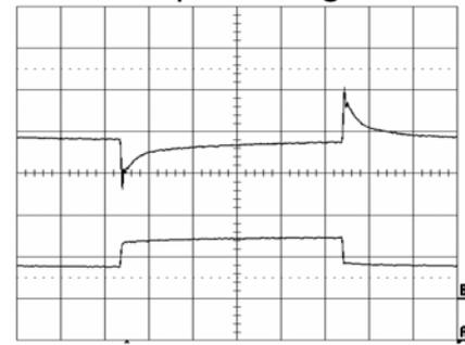
Output voltage response to load current step-
