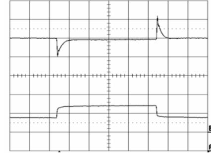
Output voltage response to load current step-
