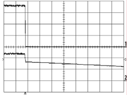
Shut-down enabled by disconnecting  $V_i$  at:
