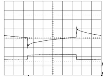
Output voltage response to load current step-
