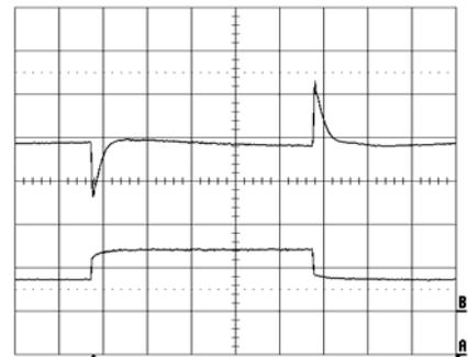
Output voltage response to load current step change (13-26-13 A) at:
