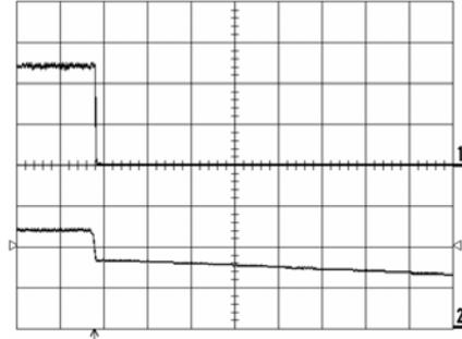
Shut-down enabled by disconnecting  $V_i$  at:
