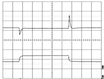
Output voltage response to load current step-
