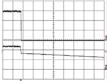
Shut-down enabled by disconnecting  $V_i$  at:
