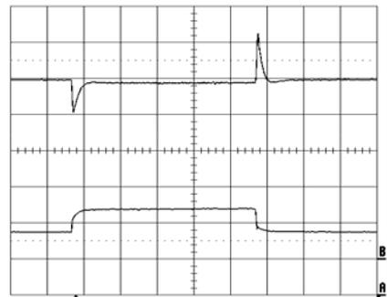
Output voltage response to load current step-
