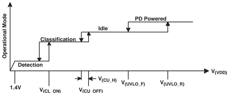
Figure 19. Threshold Voltages
