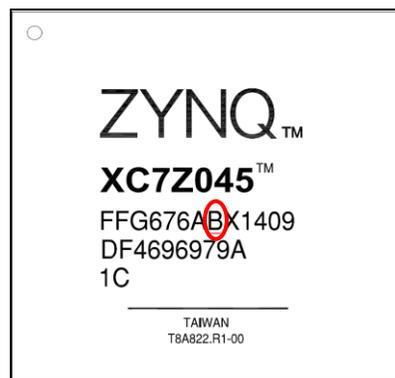
Figure 2: Top Mark for TSMC Fab 15
