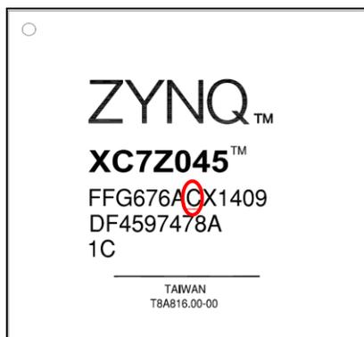
Figure 1: Top Mark for TSMC Fab 12
