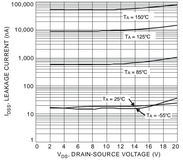
Fig. 10 Typical Leakage Current vs. Drain-Source Voltage
