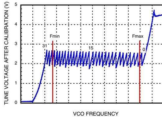
**Typical VCO Sensitivity vs. Cap @  $F_o$  Voltage**
