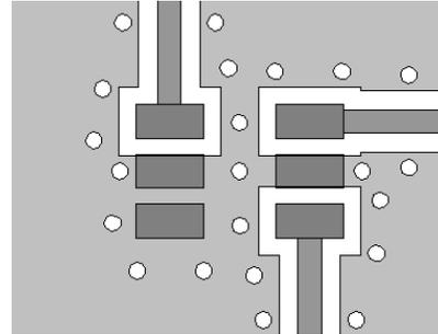
10. Recommended PCB layout shown above uses 1.6 mm FR4, grounded coplanar wave guide, transmission line width 0.70 mm and gap 0.57 mm.
