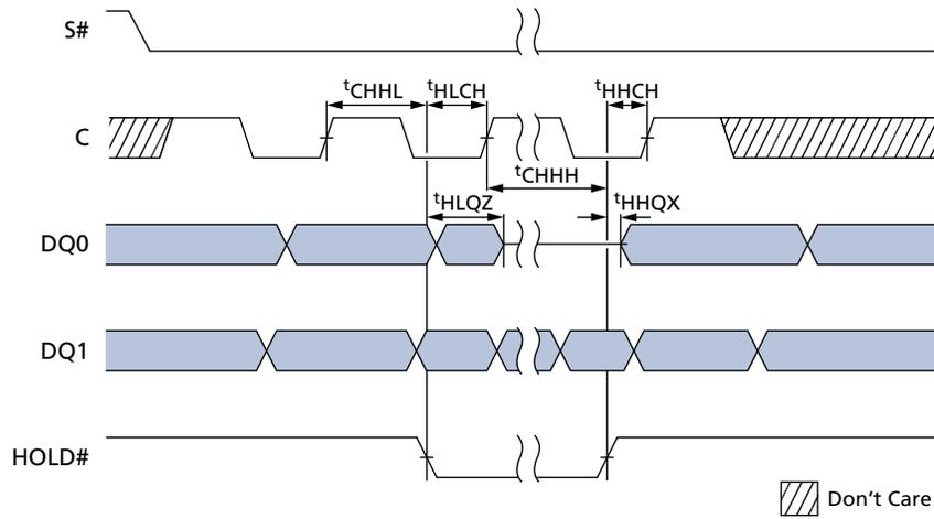
Figure 39: Output Timing
