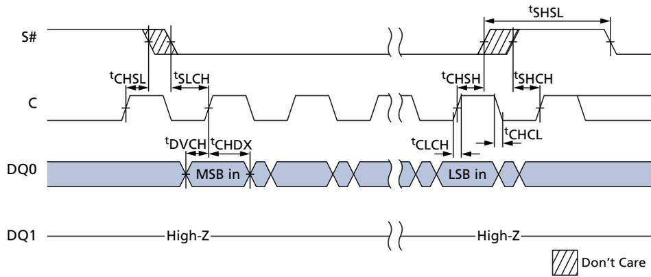
**Figure 37: Write Protect Setup and Hold During WRITE STATUS REGISTER Operation (SRWD = 1)**
