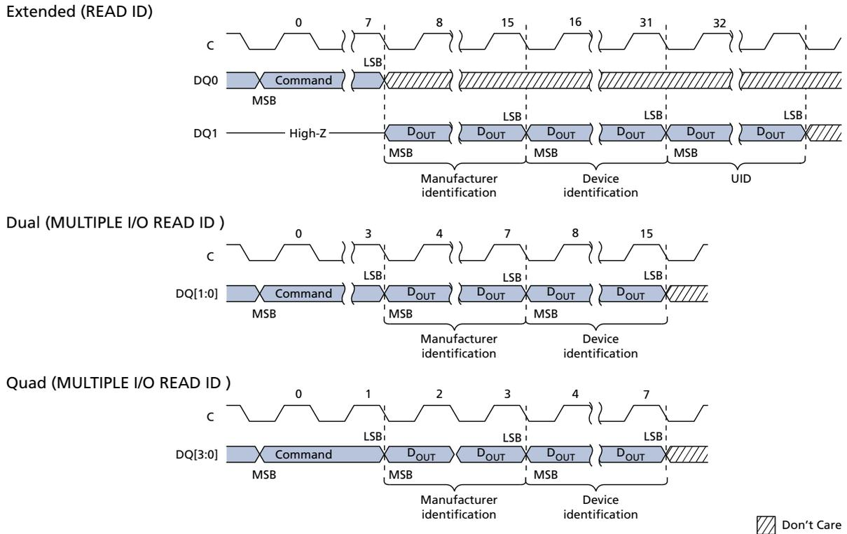
Note: 1. The READ ID command is represented by the extended SPI protocol timing shown first. The MULTIPLE I/O READ ID command is represented by the dual and quad SPI protocols as shown below extended SPI protocol.
