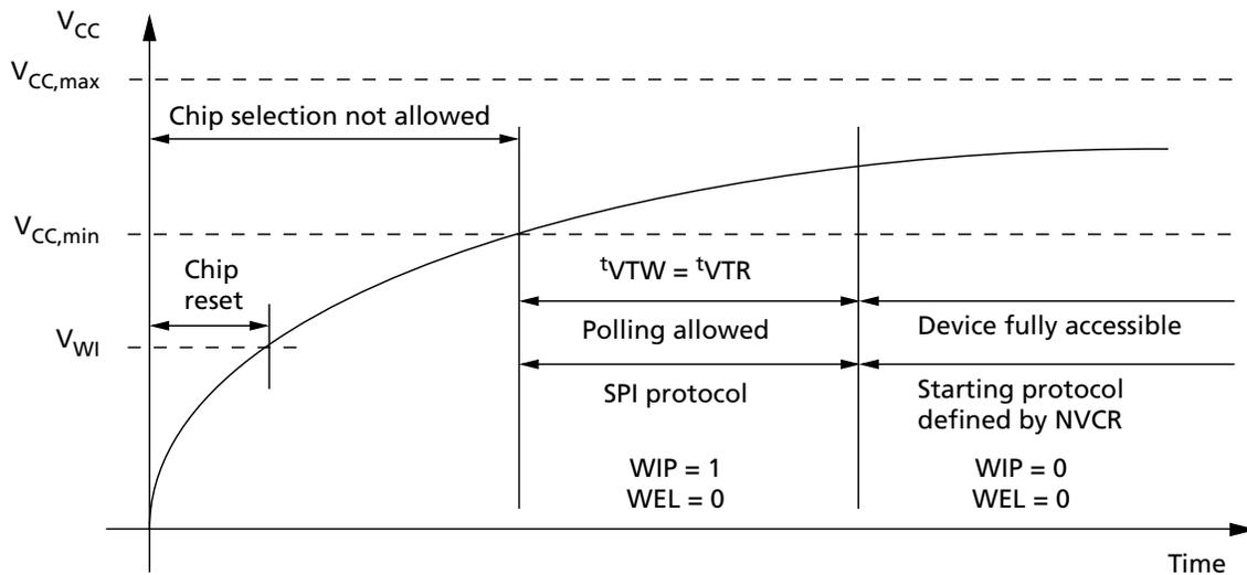
**Table 30: Power-Up Timing and V<sub>WI</sub> Threshold**
