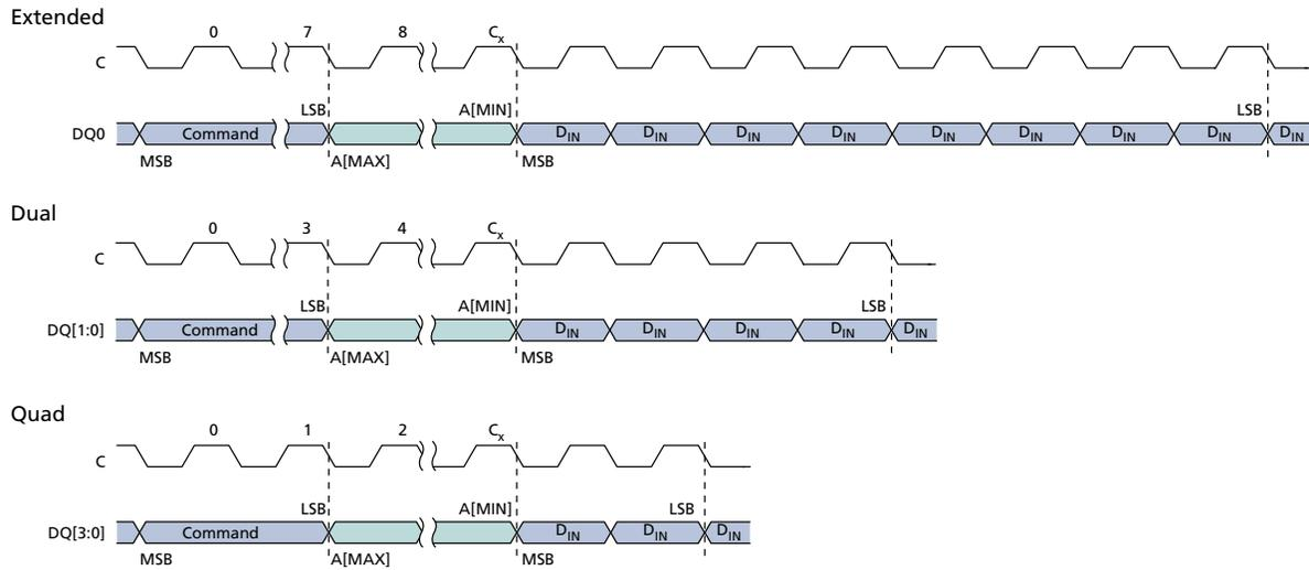
Note: 1. For extended SPI protocol,  $C_x = 7 + (A[\text{MAX}] + 1)$ .
