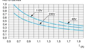
AC15control of electromagnetic loads > 72 VA, make:  $\cos \varphi$  = 0.7, break:  $\cos \varphi$  = 0.4.
