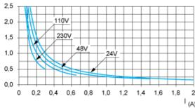
AC14control of small electromagnetic loads  $\leq$  72 VA, make:  $\cos \varphi = 0.3$ , break:  $\cos \varphi = 0.3$ .
