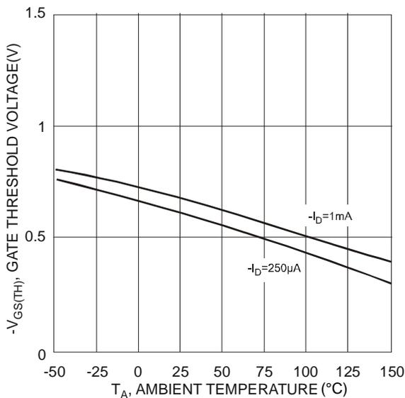
Fig. 19 Gate Threshold Variation vs. Ambient Temperature
