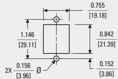
Panel Mounting Detail, Two Pole, One Handle
