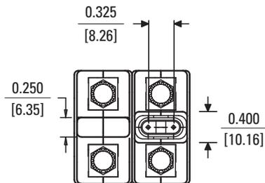
Auxiliary switch wires not shown for clarity
