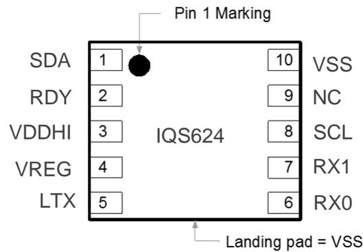
Figure 1.1 Pin out of IQS624 DFN (3X3)-10 package.
