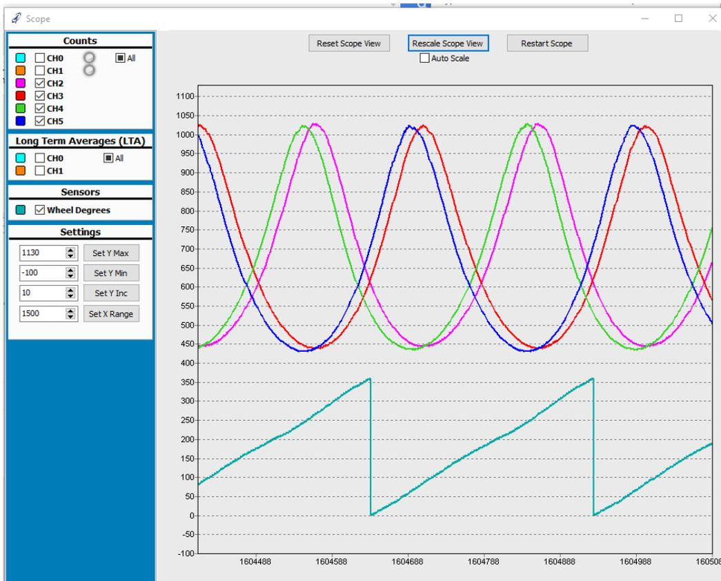
Experimentally, jog the XYZ alignment of the magnet relative to the IC and perform at least one full rotation of the magnet, assess the peaks of the channels; repeat this until all channels have approximately the same amplitude.
