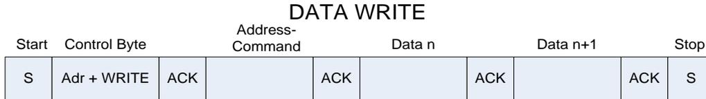
Figure 8.4 I<sup>2</sup>C Write
