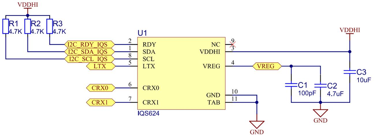
Figure 1.3 IQS624 reference schematic
