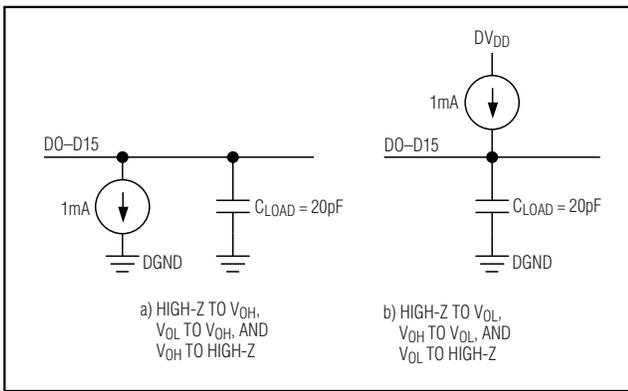
Figure 1. Load Circuits
