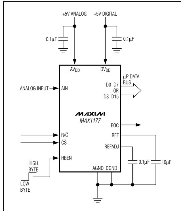
Figure 3. Typical Operating Circuit for the MAX1177
