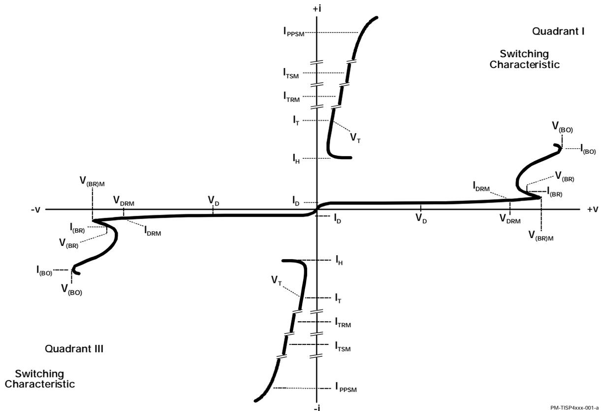
Figure 1. Voltage-Current Characteristic for T and R Terminals
