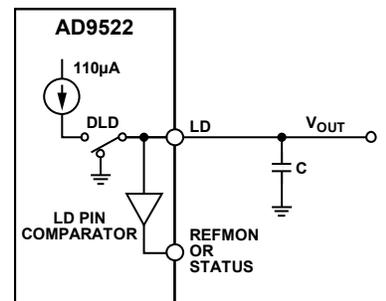
Figure 46. Current Source Digital Lock Detect
