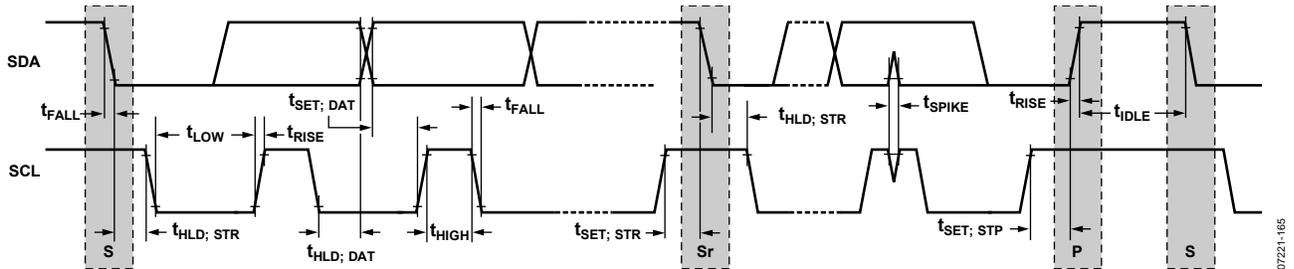
Figure 62. I<sup>2</sup>C Serial Port Timing
