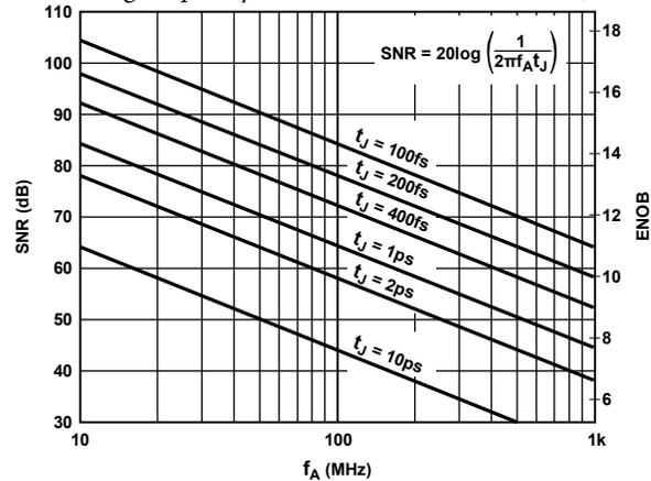
Figure 71. SNR and ENOB vs. Analog Input Frequency
