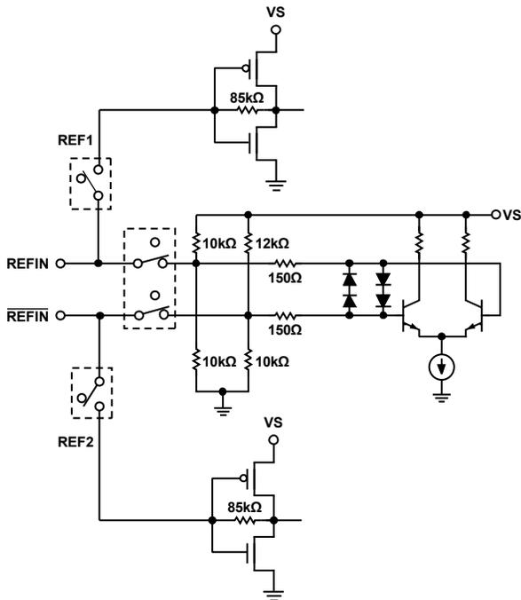
Figure 44. REF1N Equivalent Circuit for NonXTAL Mode
