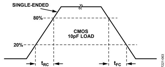
Figure 4. CMOS Timing, Single-Ended, 10 pF Load
