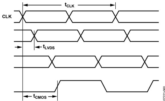
Figure 2. CLK/ $\overline{CLK}$  to Clock Output Timing, DIV = 1
