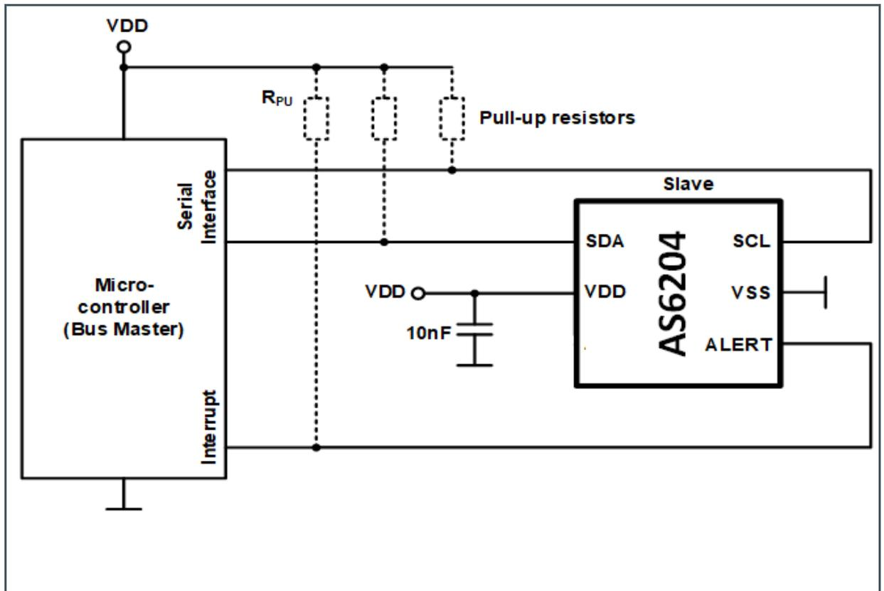
In Figure 33 the connections of the AS6204 temperature sensors to a microcontroller and the supply voltage are shown.
