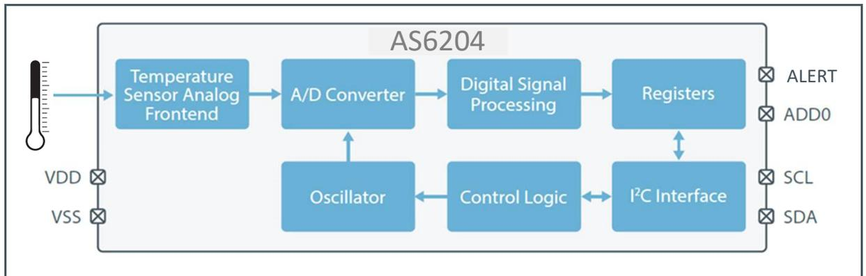
In Figure 2 the functional blocks are depicted. The sensing element for sensing the temperature is a Si bipolar transistor. The analog signal of the sensing element is converted into a digital signal by the A/D converter and the signal is further processed by a digital signal processor and written into the registers. The registers can be accessed via the serial bus interface (I<sup>2</sup>C bus).
