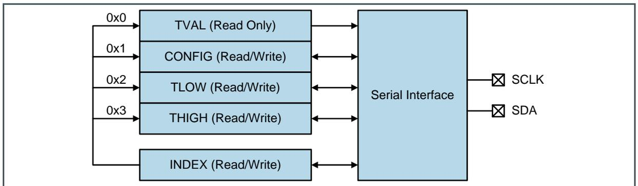
In Figure 8 the registers that the device contains are shown.
