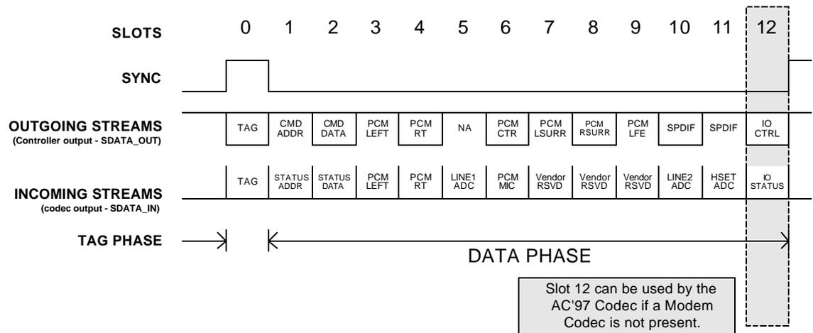
Note: The DAC & ADC can be assigned to slots 3&4, 6&9, 7&8, or 10&11.
