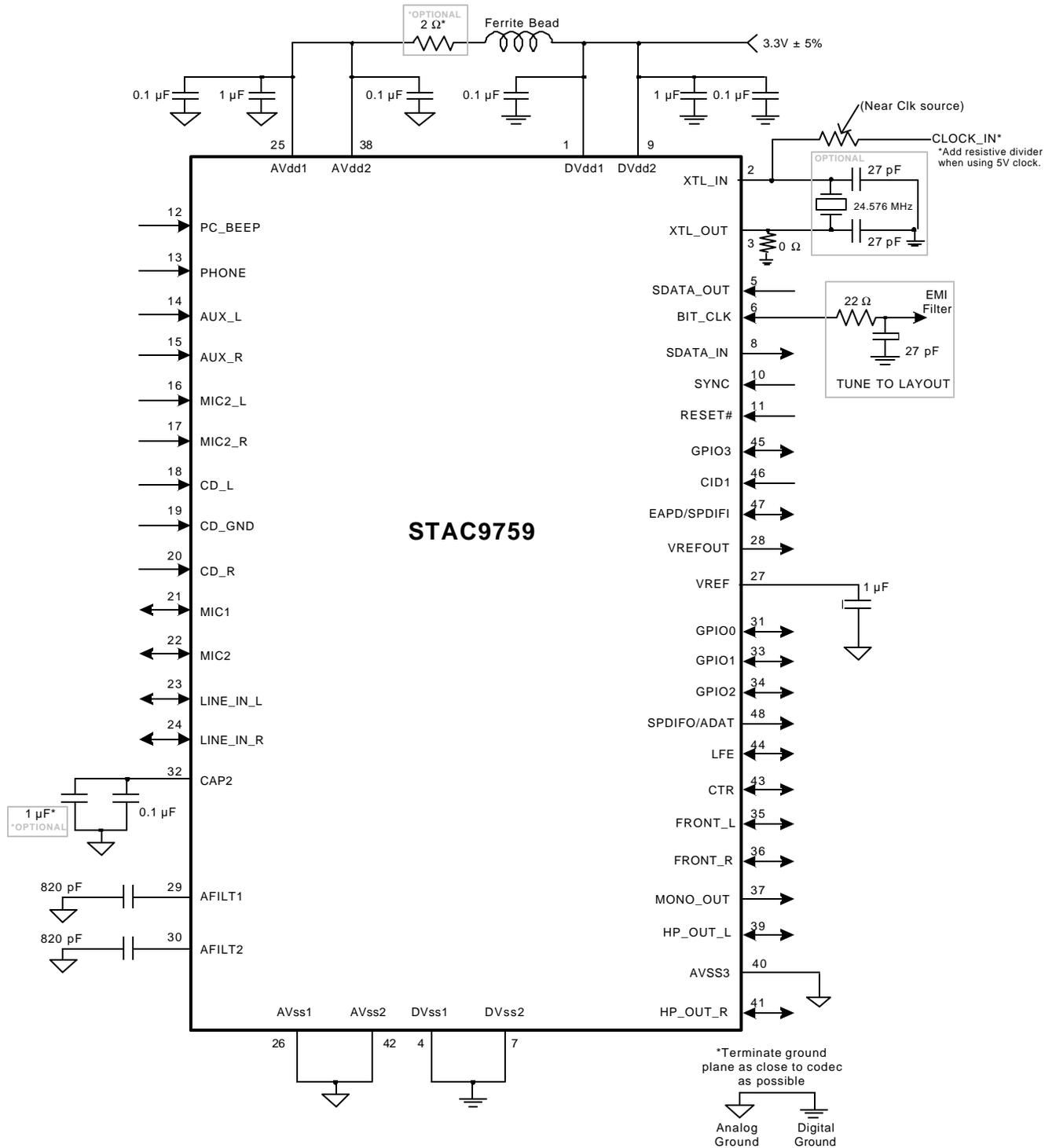
**NOTE:** If pin 48 is held high at powerup, register 28h (Extended Audio ID), bit [2] will be held to zero, to indicate the SPDIF is not available. Tie pin 48 to ground with a 10 KΩ resistor to ensure SPDIF is enabled.
