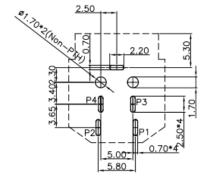
Recommended PCB Layout Top View
