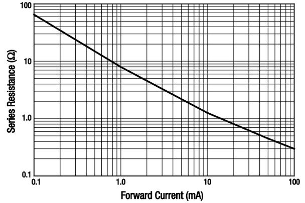
Figure 2. Series Resistance vs Forward Current @ 100 MHz
