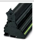
Fuse modular terminal block, fuse type: Glass / ceramics / ..., connection method: Screw connection, cross section:  $0.14 \text{ mm}^2$ -  $6 \text{ mm}^2$ , AWG: 26 - 10, nominal current: 28 A, nom. voltage: 24 V, width: 6.2 mm, fuse type: G /  $5 \times 20$ , mounting type: NS 35/7,5, NS 35/15, color: black
