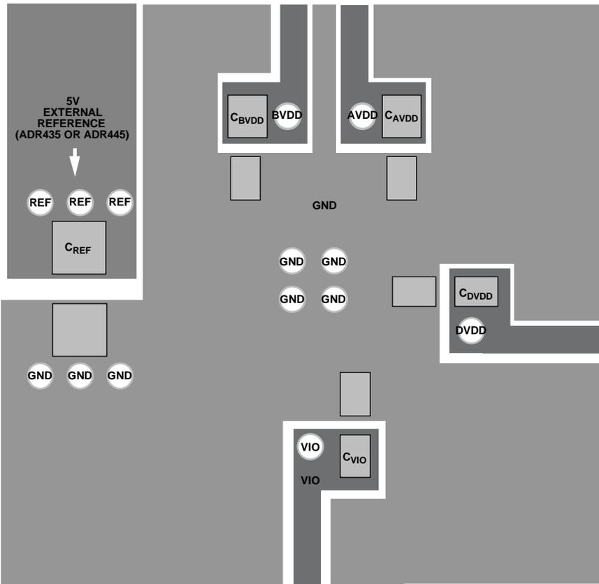
Figure 39. Example Layout of the AD7985 (Bottom Layer)
