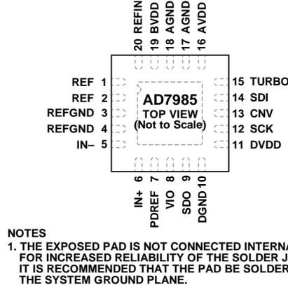
Figure 4. Pin Configuration
