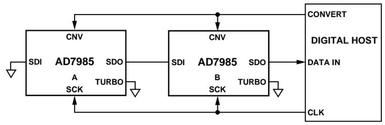
Figure 34. Chain Mode Without Busy Indicator Connection Diagram
