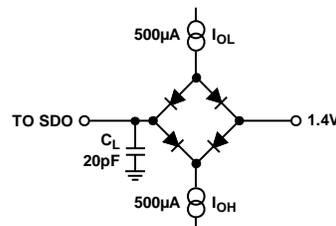
Figure 2. Load Circuit for Digital Interface Timing
