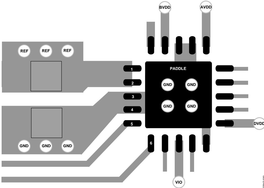
Figure 38. Example Layout of the AD7985 (Top Layer)
