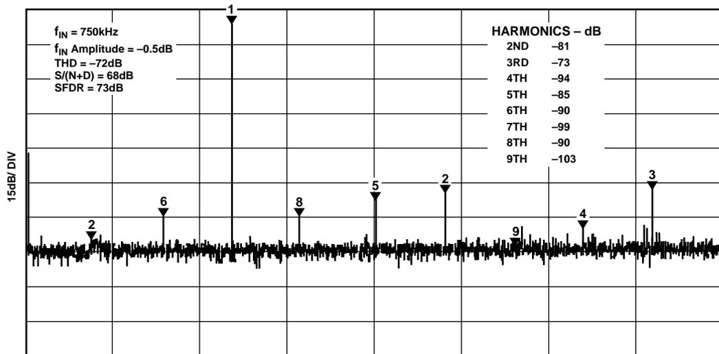
Figure 6. AD871 Typical FFT,  $f_{IN} = 750$  kHz
