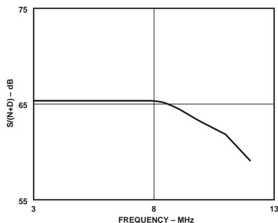
Figure 27. Typical  $S/(N+D)$  vs. Clock Frequency
