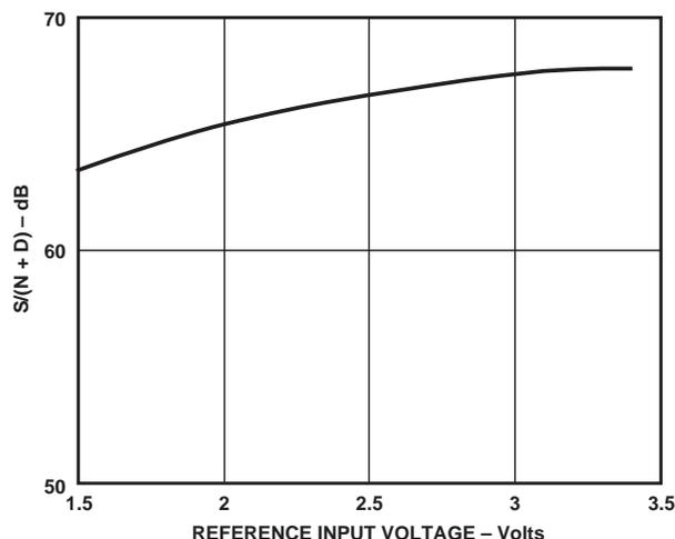
Figure 20. S/(N+D) vs. Reference Input Voltage,  $f_{IN} = 1\text{ MHz}$ ,  $FS = 5\text{ MHz}$
