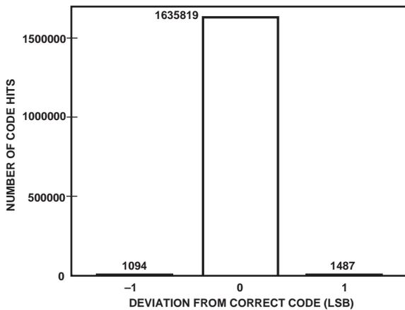
Figure 8. AD871 Output Code Histogram for DC Input
