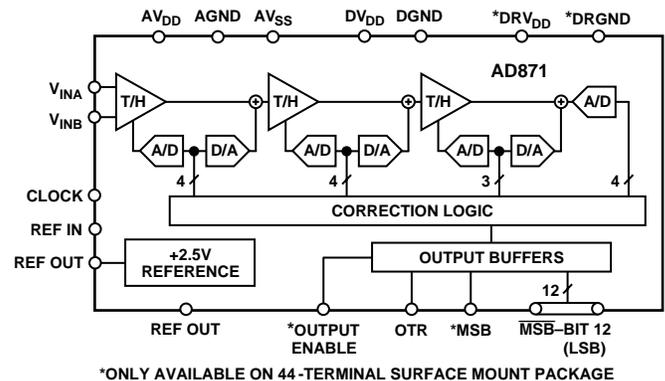
The AD871 is fabricated on Analog Devices' ABCMOS-1 process, which uses high speed bipolar and CMOS transistors on a single chip. High speed, precision analog circuits are now combined with high density logic circuits.
