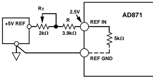
Figure 21. Optional +5 V Reference Input Circuit
