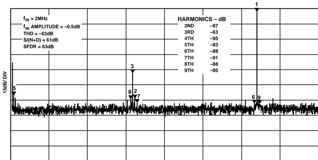
Figure 7. AD871 Typical FFT,  $f_{IN} = 2$  MHz
