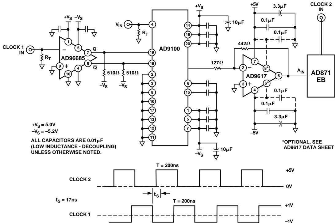
Figure 33. Undersampling Using the AD871 and AD9100
