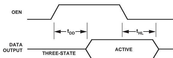
Figure 25. Three-State Output Timing Diagram
