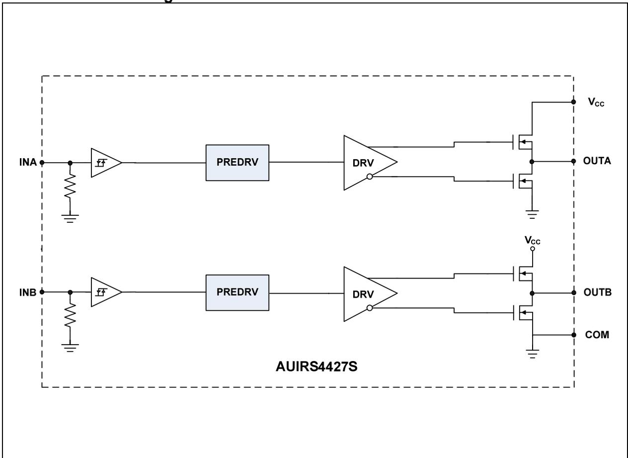
**Input/Output Pin Equivalent Circuit Diagrams**
