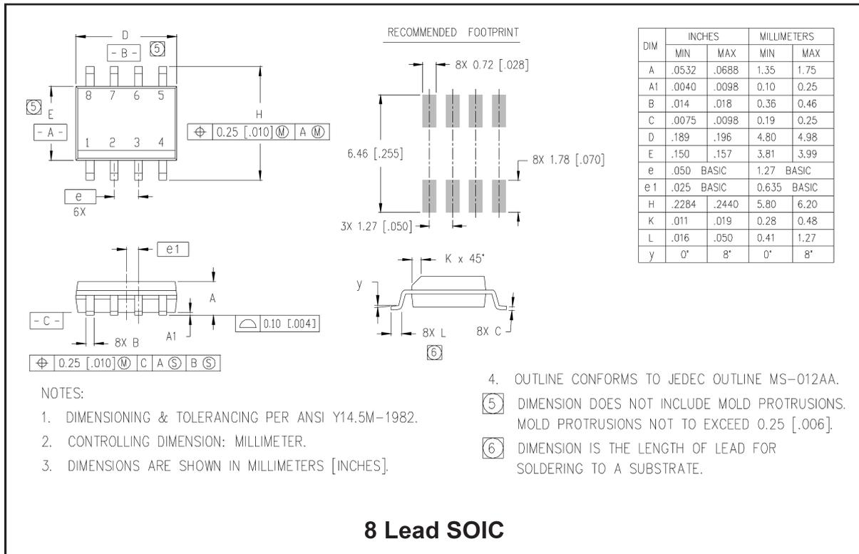
**Package details: SOIC8N, Tape and Reel**
