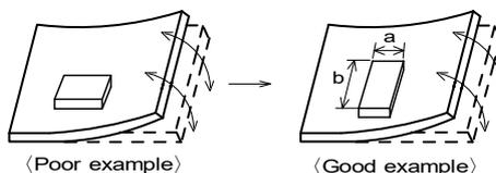
(2) Components location on PCB separation
