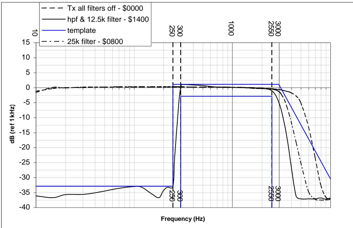
Figure 9 Tx Channel Audio Filter Response and Template (TIA)
