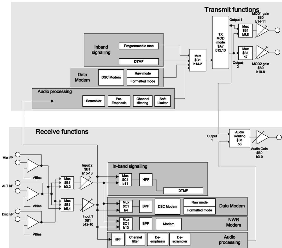
Figure 5 Signal Routing
