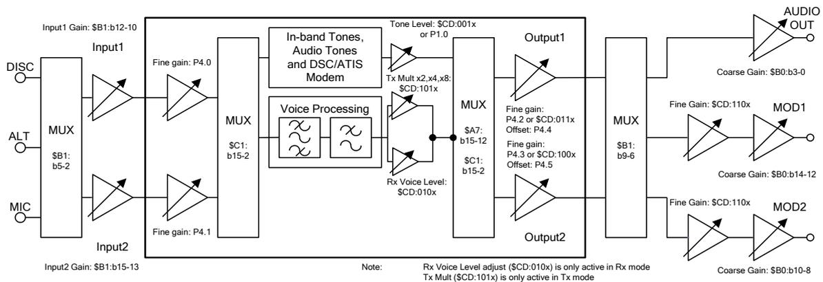
Figure 14 Level Adjustments
