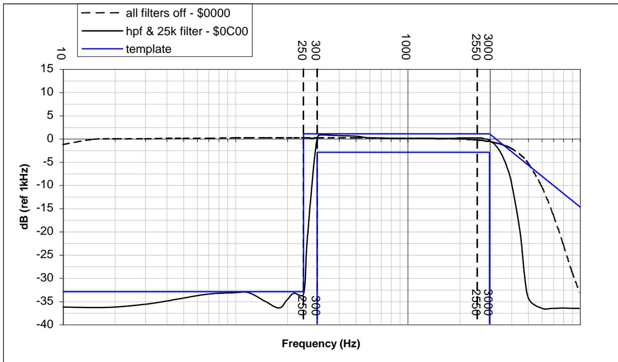
Figure 6 Rx 25kHz Channel Audio Filter Frequency Response
