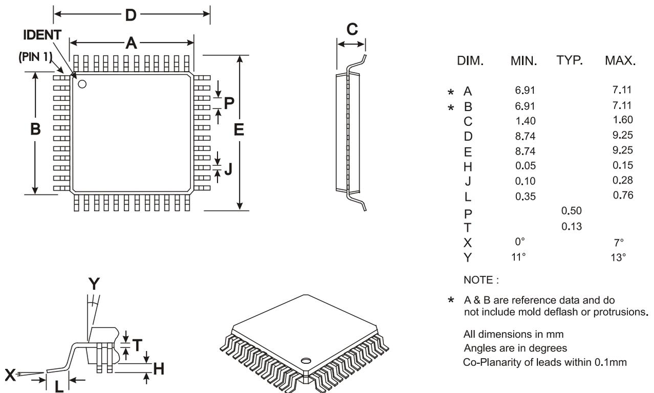
Figure 22 Mechanical Outline of 48-pin LQFP (L4)
