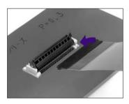
C)Push the lock lever down, by rotating the lever inward.
