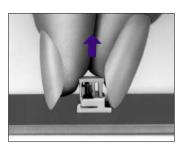
B)Insert the FFC/FPC conductor surface upside down. Insert the FFC/FPC diagonally from above the connector until it firmly hooks on the positioning point. Slightly push the FFC/FPC, and check that it has been retained to the positioning point.
