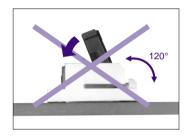
C)Make certain to fully insert the FFC/FPC into the connector. Improper insertion causes the FFC/FPC to be disconnected, or conductivity failure.
