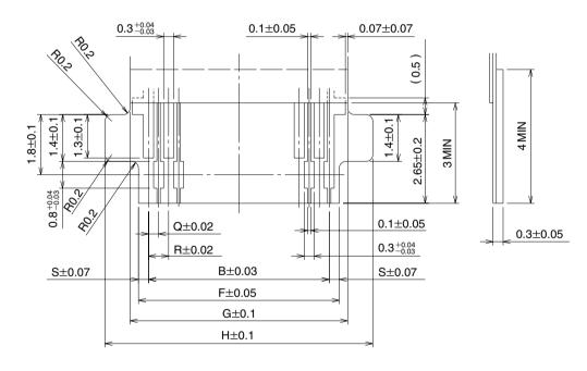
\* Forced film material shall be polyamide + thermal hardened additives.
