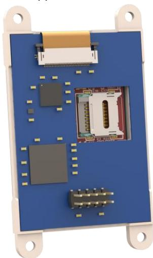
The micro-SD socket is a latch type, so it is accessible from the top, rather than a push/push or push/pull style which is accessible from the side.
