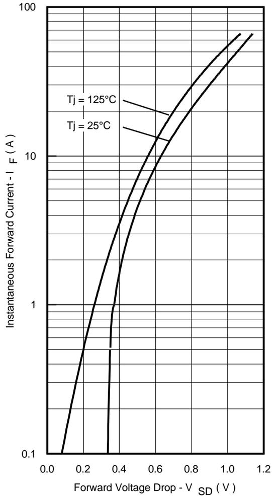
Fig. 11 - Typical Forward Voltage Drop Characteristics
