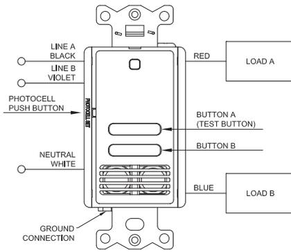
FIGURE 4 - MULTI-TECH, SINGLE CIRCUIT,
