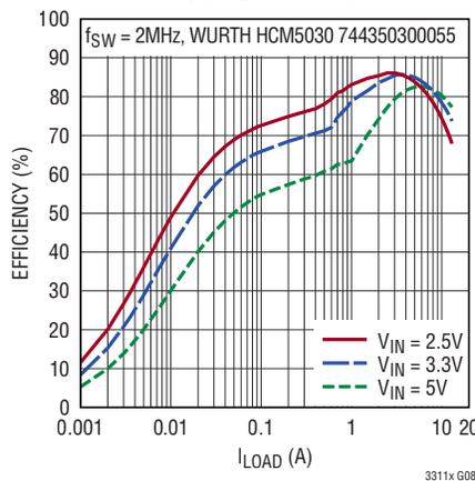
**Efficiency,  $V_{OUT} = 1.2V$**
