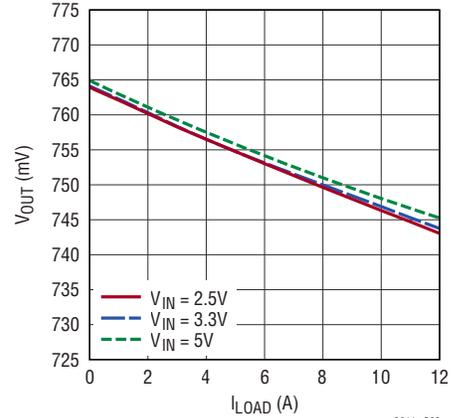
**$V_{OUT}$  Load Regulation**
