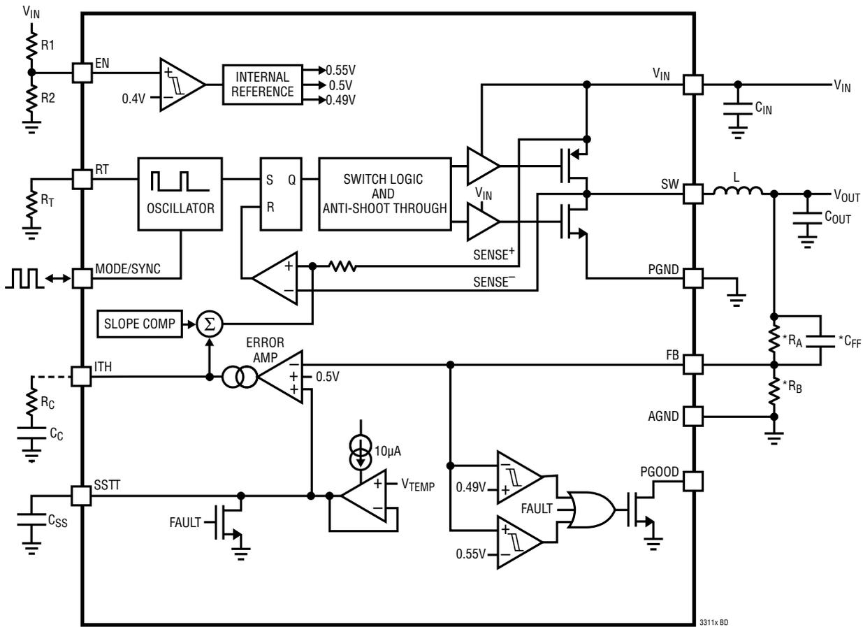
\*ON THE LTC3311-X, THE  $R_A$  AND  $R_B$  RESISTORS ARE INTERNAL, ALONG WITH  $C_{FF}$
