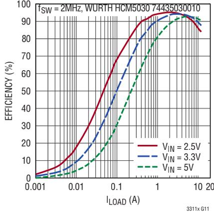
**Efficiency,  $V_{OUT} = 1.8V$
