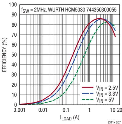
**Efficiency,  $V_{OUT} = 0.5V$**
