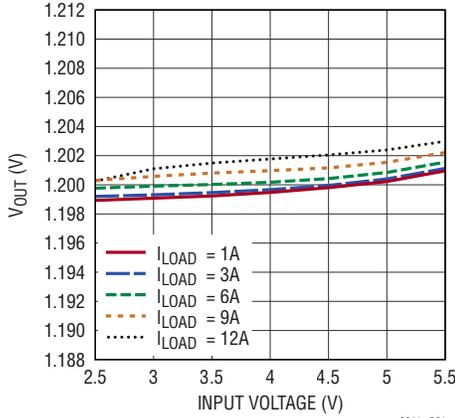
**$V_{OUT}$  Load Regulation**
