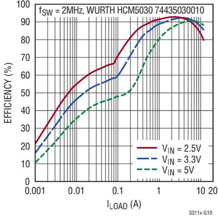
**Efficiency,  $V_{OUT} = 1.8V$
