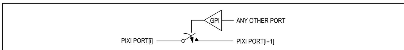
Figure 11. PIXI Ports as a Controllable Analog Switch
