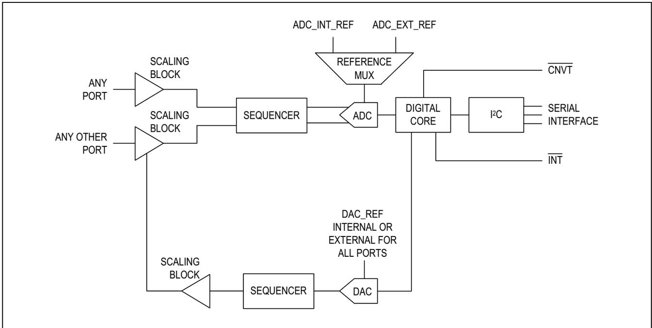
Figure 4. ADC with Pseudo-Differential Input Set by DAC
