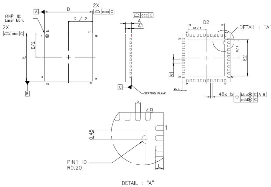
**Figure 2.1. 7 x 7 mm 48-pin QFN**
