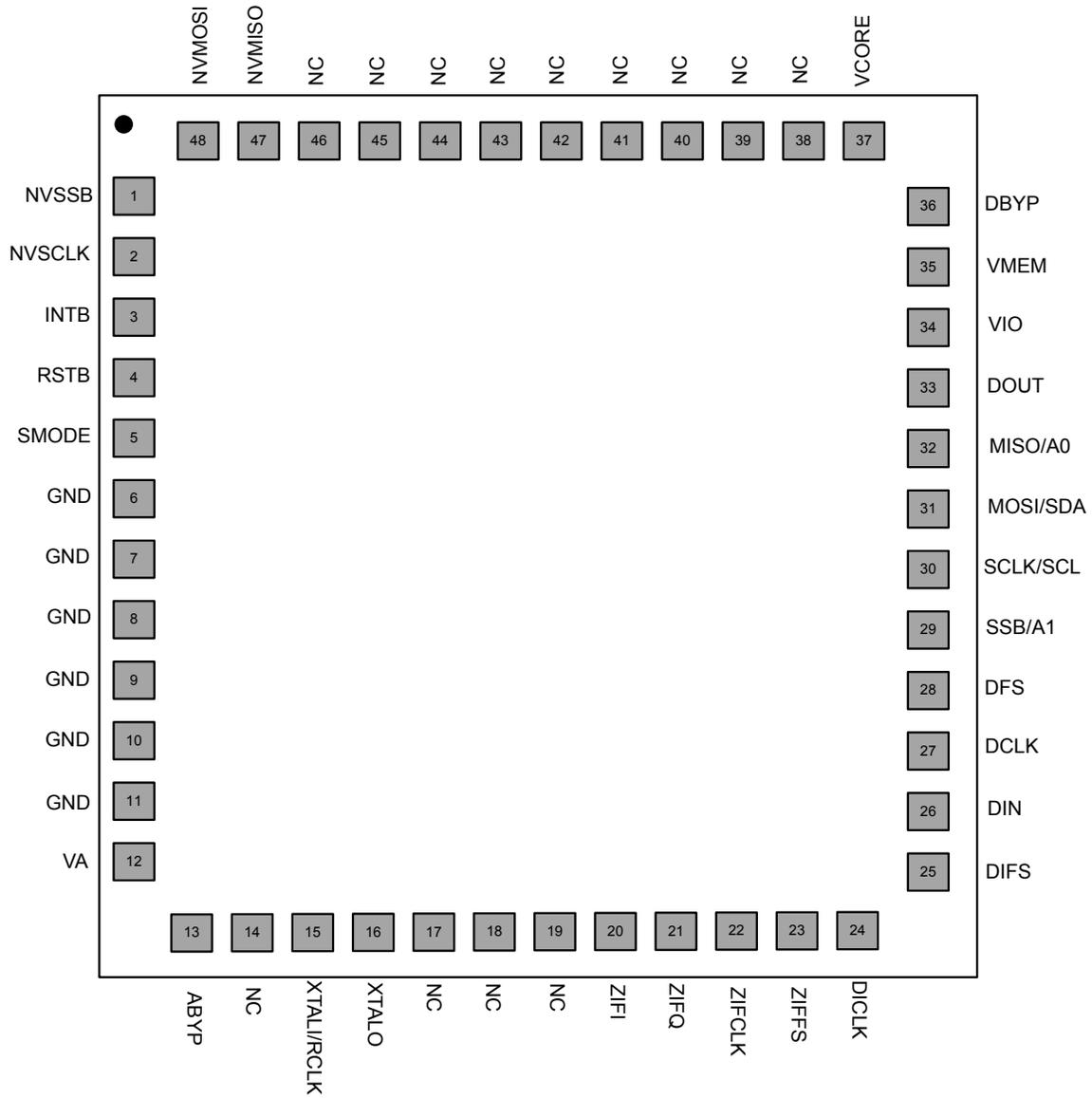
Figure 1.1. 48-pin QFN
