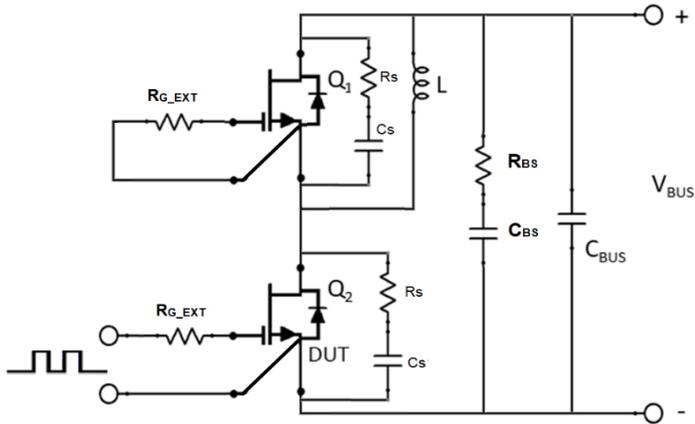
Figure 29. Schematic of the half-bridge mode switching test circuit. Note, a bus RC snubber ( $R_{BS} = 1\Omega$ ,  $C_{BS} = 100\text{nF}$ ) is used to reduce the power loop high frequency oscillations.
