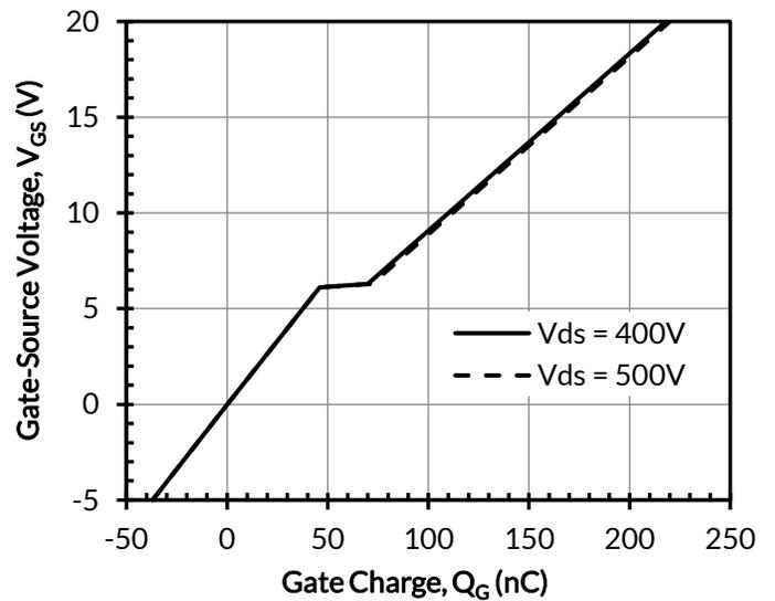
Figure 8. Typical gate charge at  $I_D = 80A$
