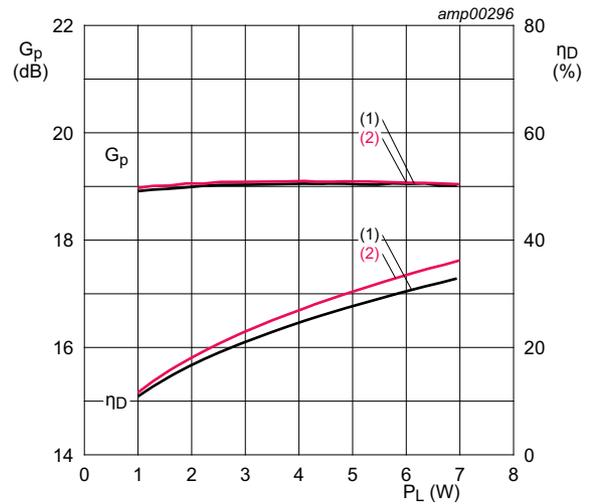
$V_{DS} = 28$  V;  $I_{Dq} = 180$  mA.
