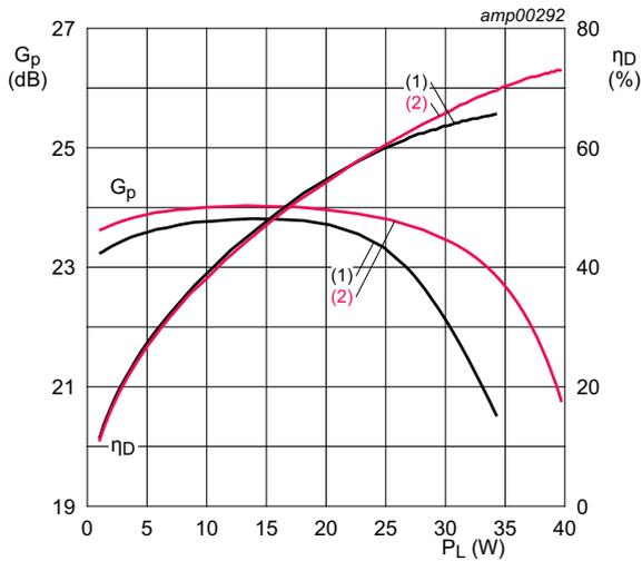
$V_{DS} = 28\text{ V}; I_{Dq} = 180\text{ mA}.$
