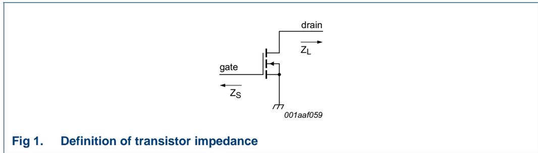
Fig 1. Definition of transistor impedance
