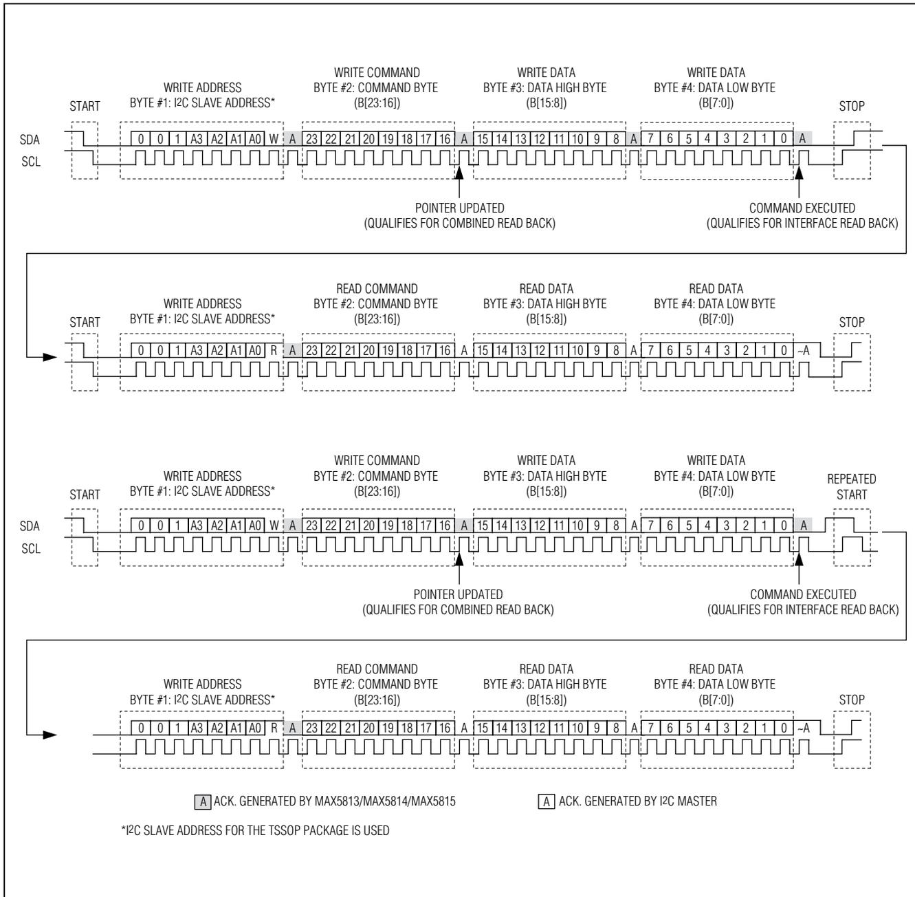
Figure 7. Interface Verification I<sup>2</sup>C Register Read Sequences
