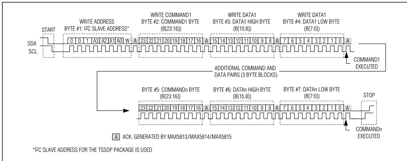
Figure 5. Multiple Register Write Sequence (Standard I<sup>2</sup>C Protocol)
