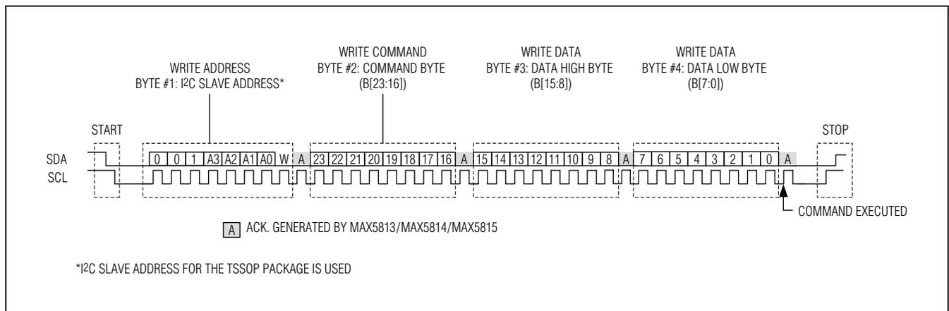
Figure 4. I<sup>2</sup>C Single Register Write Sequence
