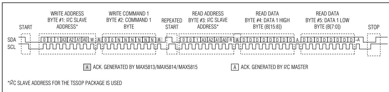
Figure 6. Standard I<sup>2</sup>C Register Read Sequence
