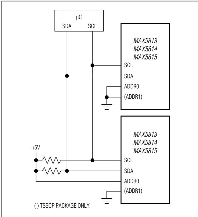
Figure 8. Typical I<sup>2</sup>C Application Circuit
