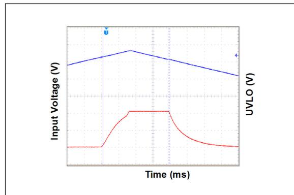
**FIGURE 2-24:** Undervoltage Lockout.
