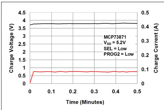
**FIGURE 2-26:** Complete Charge Cycle (130 mAh Li-Ion Battery).
