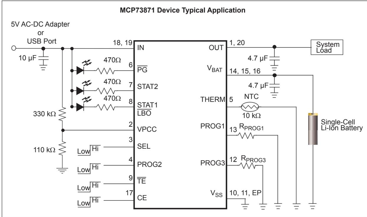
**FIGURE 6-1:** MCP73871 Typical Stand-Alone Application Circuit with VPCC.
