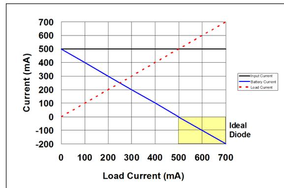
FIGURE 4-4: Input Current Limit Control - USB Port.
