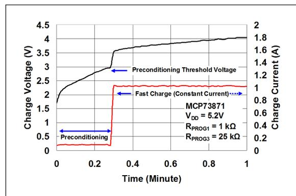
**FIGURE 2-28:** Typical Charge Profile in Preconditioning (1000 mAh Battery).
