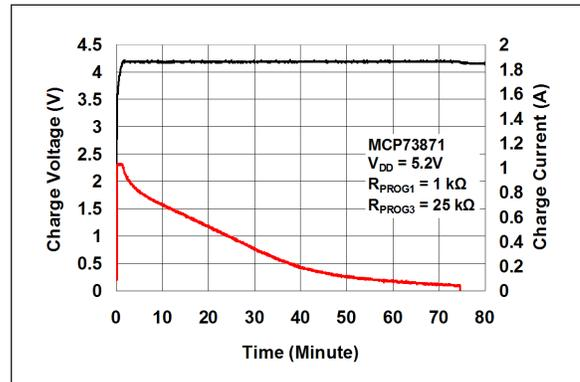
**FIGURE 2-27:** Complete Charge Cycle (1000 mAh Li-Ion Battery).
