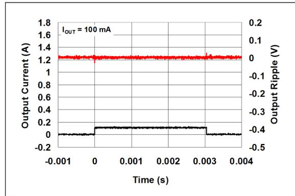
**FIGURE 2-22:** Load Transient Response.  $I_{OUT} = 100\text{ mA}$ .
