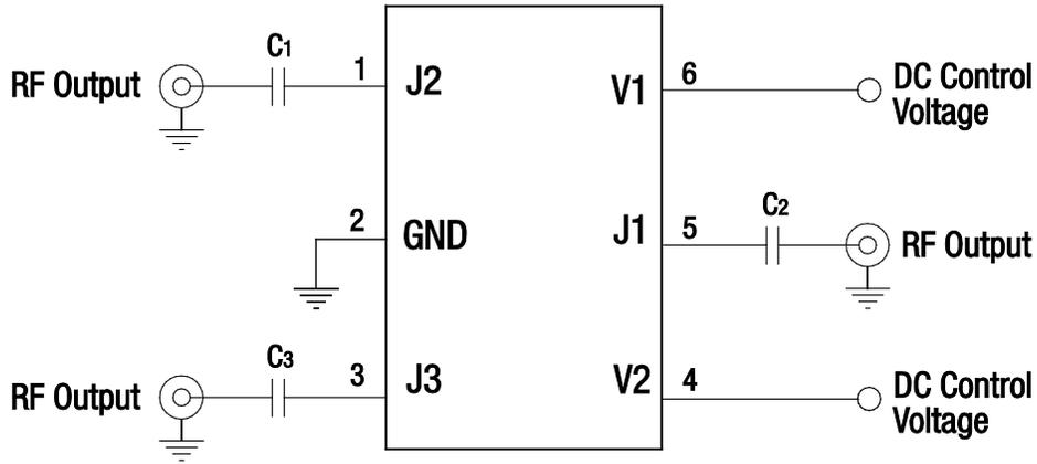
*Note: Use 47 pF blocking capacitors (C1, C2, C3) for >500 MHz operation. Higher values recommended for lower frequency operation. Exposed paddle must be grounded.*
