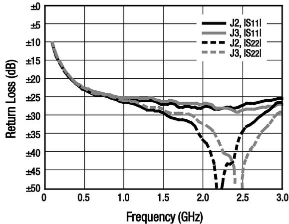
Figure 5. Return Loss vs Frequency (Insertion Loss State)
