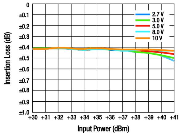
Figure 6. Insertion Loss vs Input Power (@ 900 MHz)
