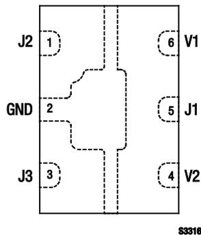
**Figure 2. SKY13290-313LF Pinout –6-Pin QFN (Top View)**
