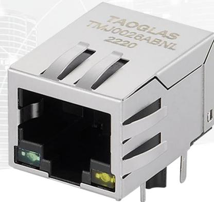
Featuring a popular footprint and compatible package to industry RJ45 Integrated Connectors standards, the Taoglas TMJ0026ABNL is an RJ45 Integrated Connector 10/100Base-T Single Port Tab Down with EMI Finger, its shielded short body design offers extra space, and with a schematic that enables Auto Transformer feature that will provide better EMI performance.
