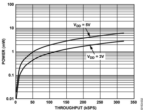
Figure 32. Power vs. Throughput Rate for Power-Down Mode
