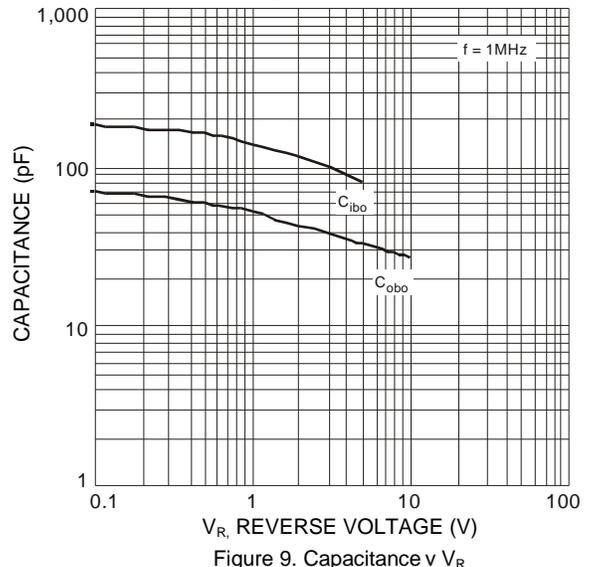
Figure 9. Capacitance v  $V_R$
