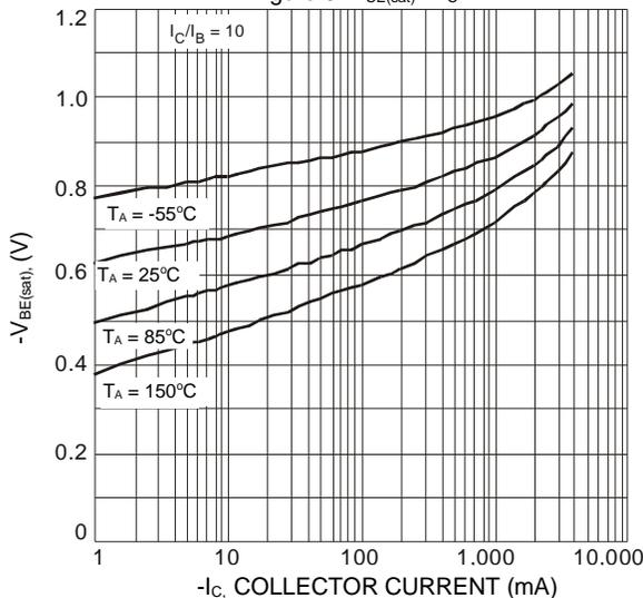
Figure 8.  $V_{BE(sat)}$  v  $I_C$
