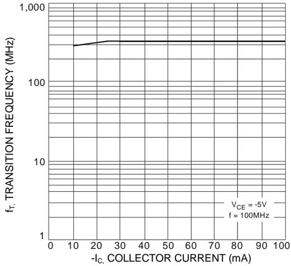
Figure 10. f<sub>T</sub> v I<sub>C</sub>
