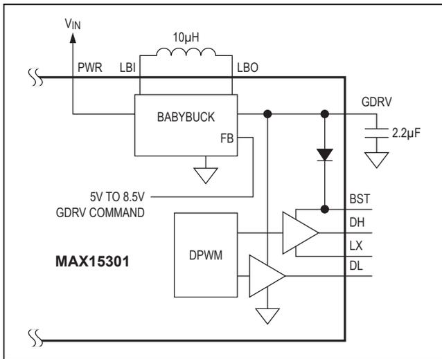
Figure 10. Gate Drivers Powered by Switching Regulator
