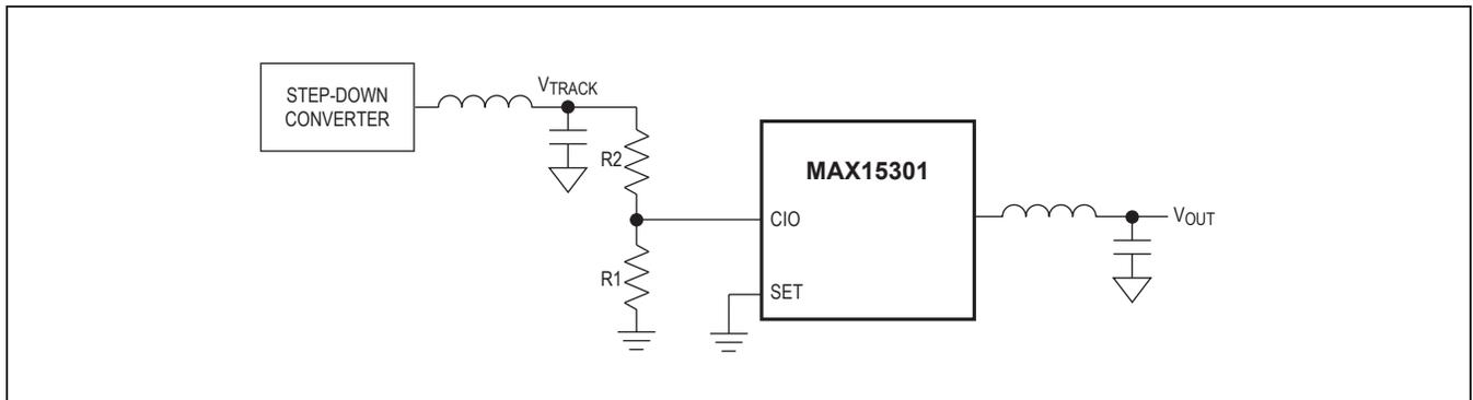
Figure 5. Tracking Mode Configuration
