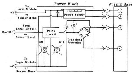
Figure 4. RPBA & RPBA-1—Wiring Diagram
