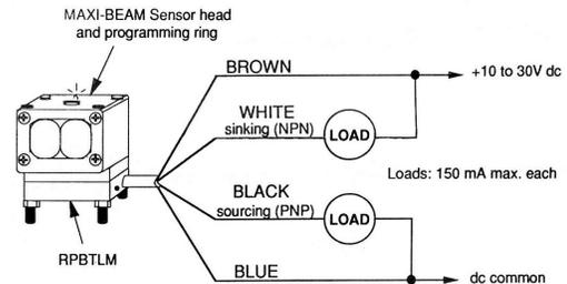
The RPBTLM powers the sensor head from a 10 V dc to 30 V dc supply. It contains output circuitry to allow an interface of the signal from the sensor head to a load or to a logic input.
