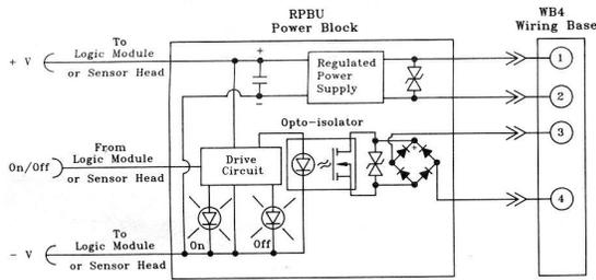
Figure 14. RPBU—Wiring Diagram
