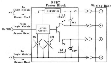
Figure 2. RPBT and RPBT-1—Wiring Diagram
