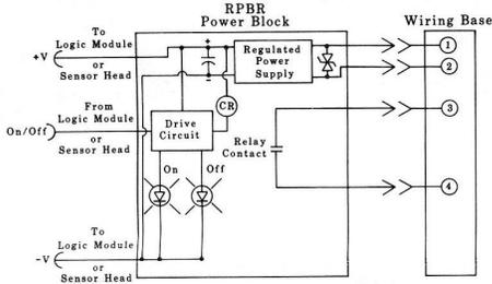
Figure 10. RPBR—Wiring Diagram
