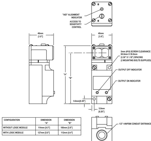
Figure 18. Dimensions for the FF models
