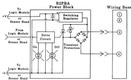
Figure 8. R2PBA & R2PBB—Wiring Diagram
