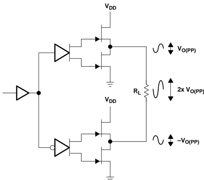
**Figure 23. Bridge-Tied Load Configuration**
