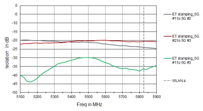
Isolation between each of the three antennas is below -20dB.
