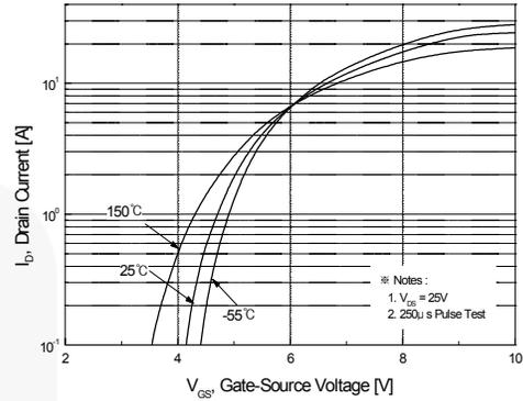
Figure 2. Transfer Characteristics
