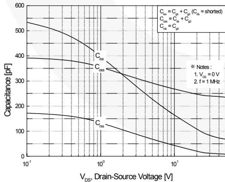
Figure 5. Capacitance Characteristics
