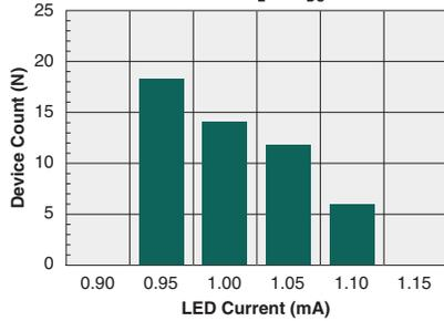
Typical  $I_F$  for Switch Dropout
